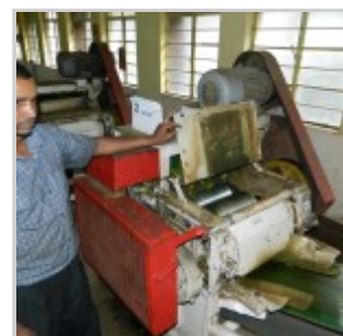
The second cut, where tea leaves are grounded
