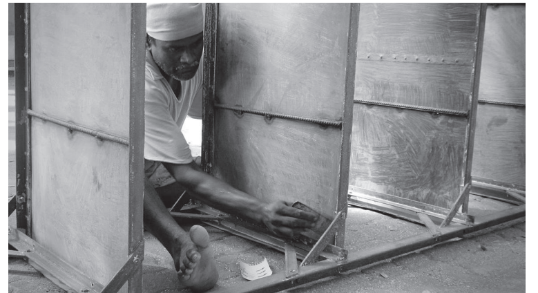
A worker sanding iron panels. To me, there was a beauty beyond the rough work he was engaged in.
